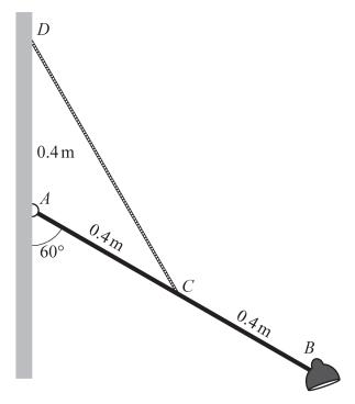
The diagram shows a wall-mounted light. It consists of a rod AB of mass 0.25 kg and length 0.8 m which is freely hinged to a vertical wall at A, and a lamp of mass 0.5 kg fixed at B. The system is held in equilibrium by a chain CD whose end C is attached to the midpoint of AB. The end D is fixed to the wall a distance 0.4 m vertically above A. The rod AB makes an angle of  $60^{\circ}$  with the downward vertical.
