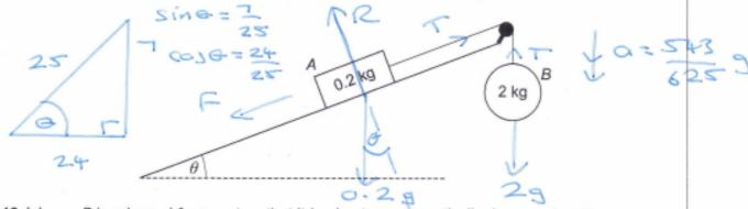
18 (a) B is released from rest so that it begins to move vertically downwards with an acceleration of  $\frac{543}{625}$  g m s<sup>-2</sup>
