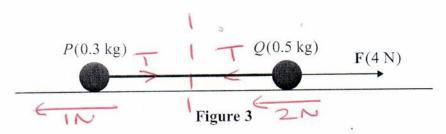
Two particles P and Q, of mass 0.3 kg and 0.5 kg respectively, are joined by a light horizontal rod. The system of the particles and the rod is at rest on a horizontal plane. At time t=0, a constant force F of magnitude 4 N is applied to Q in the direction PQ, as shown in Figure 3. The system moves under the action of this force until t=6 s. During the motion, the resistance to the motion of P has constant magnitude 1 N and the resistance to the motion of Q has constant magnitude 2 N.
