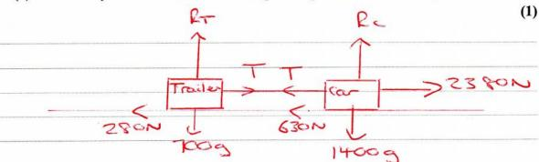
a) For car + trailer  $R(\rightarrow)$   $(70^{\circ}+14^{\circ}) \times a = 2380-630-280$ 2100 a = 1470
